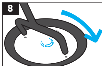
8 Insert new cartridge into housing and turn key to right (clockwise) to lock and click into place.
