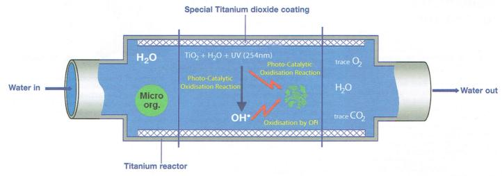
The Rodin Titanium Advanced Oxidation Process (AOP) is an environmentally friendly 'gatekeeper' solution that prevents Legionella and other organisms from entering the water system of a building while preventing the formation of bio-films.
