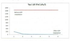
Overall the bacterial count in the hospital water was reduced by 99.9% and the AOP was able to deliver clean water into the potable water system and reduce bacteria within the hospital.
