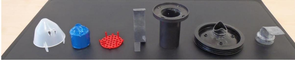
The pressed tube is both larger and thicker to the Whiffaway valve. Urimat's valve thickness was shown to reduce liquid flow rate. This valve is commonly known to be prone to sticking, for which reason Urimat uses talcum powder to help mitigate. Due to the laterally closed tube, the Urimat valve was shown to be prone to blockage from common debris.
