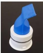
Flow rate was tested to show about half of that of the HPKV. Furthermore, the bended tube valve is very prone to sticking. When we initially tested the valves, the flaps stuck to each other and drainage time of 250 ml was longer than 30 seconds. In addition the pressed tube structure with the bend in the middle section of the membrane proved difficult to flush out common debris.
