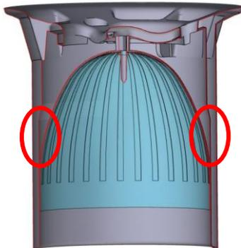
*Picture: The silicone bell (pale blue) is in a radial contact with the inner wall of the PP tubing (grey).*
