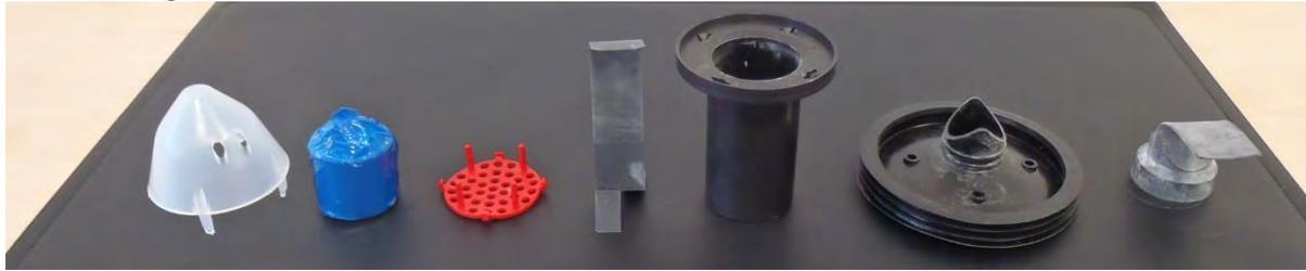
The pressed tube is both larger and thicker to the Whiffaway valve. Urimat's valve thickness was shown to reduce liquid flow rate. This valve is commonly known to be prone to sticking, for which reason Urimat uses talcum powder to help mitigate. Due to the laterally closed tube, the Urimat valve was shown to be prone to blockage from common debris.
